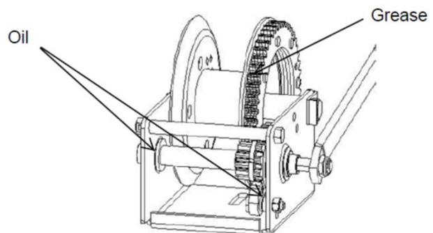
3. Check for wear on the gear teeth on the winch drum or gear on the primary shaft. If excessive replace winch. Check load being applied to winch as overloading will cause excessive wear.
